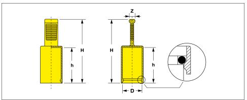
material: Flexible TPE, for an optimal clamp fit and seal
